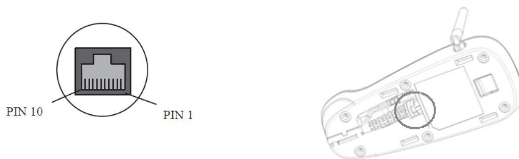
Pin assignment of CD15 connector
